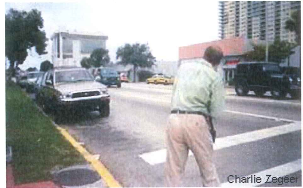
Removing parking from corners can improve visibility between pedestrians and approaching motorists.
