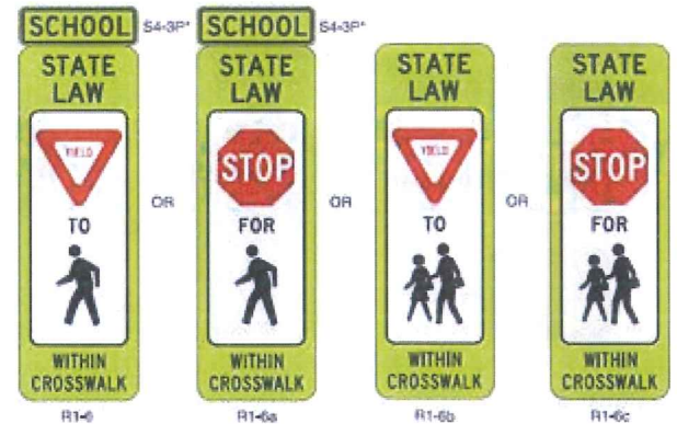
Figure 1: In-street yield and stop signs. The 2009 MUTCD added a new option to use the schoolchildren symbol rather than the pedestrian symbol when an in-street sign is used at a school crossing. Image from the 2009 MUTCD.
