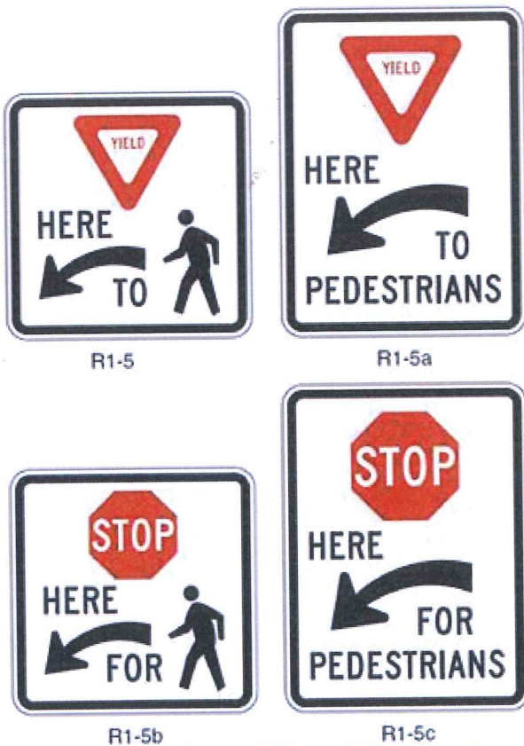
Figure 3: Examples of STOP and YIELD here to pedestrian signs. Image provided by PBIC Designing for Safety course.
